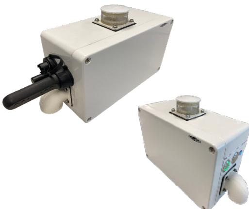
**LOAC** (Light Optical Aerosol Counter) is an aerosol counter providing a particle concentration and an average of the aerosol optical nature. This miniaturized and versatile instrument works with a laser diode and 2 detectors placed at 12° and 60° respectively, thus offering a high level of sensitivity.
