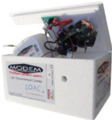
**LOAC** (Light Optical Aerosol Counter) is an aerosol counter providing a particle concentration and an average of the aerosol optical nature. This miniaturized and versatile instrument works with a laser diode and 2 detectors placed at 12° and 60° respectively, thus offering a high level of sensitivity.
