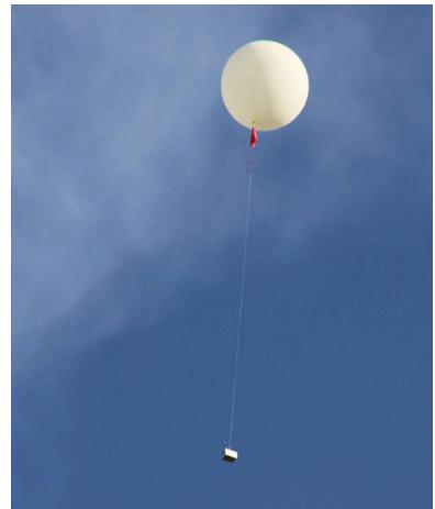
The **LOAC Telemetry** is powered by 2 alkaline batteries. It can be used under a captive balloon or weather balloon.
