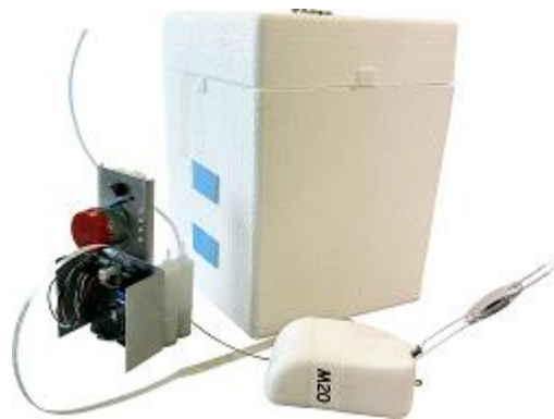
ECC Ozone sonde with Meteomodem interface for M20 radiosonde
